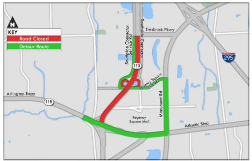
Improvements along the Southside Connector include resurfacing of the roadway, shoulder treatments, drainage, new highway signage and guardrail repairs. The Southside Connector on and off-ramps at Regency Square Boulevard North, Tredinick Parkway, Merrill Road, including the ramp to I-295 northbound, the I-295 southbound flyover and the Southside Connector Service roads will also be resurfaced.
